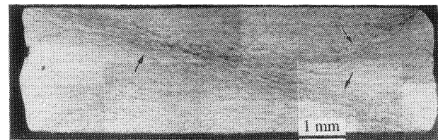
Fig. 10. Cross-section of 7.5-mm specimen deformed at room temperature and 3500 s^{-1} to a strain of -0.8 ; shear bands marked by arrows.
